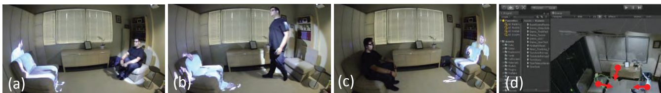
Figure 3. A sequence showing Room2Room placement capabilities: (a-c) when the local user changes their seat, Room2Room automatically remaps the remote user to the other available seat; (d) the view of that same interaction in the Unity editor, which is also used to annotate seating and standing locations (indicated with red arrows).
