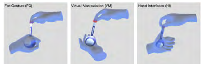
Figure 11: In this study, we explored three techniques for the interactive control scenarios, including two baselines and hand interfaces. From left to right: Fist Gesture, Virtual Manipulation, and Hand Interfaces.
