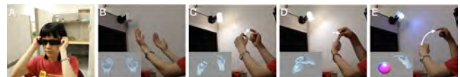
Figure 2: A user uses Hand Interfaces in concert with an AR device to quickly and easily control a smart lighting system. Specifically, the Toggle switch is used to turn on/off the light, the Joystick controls its pan/tilt, and a fist-imitated Color palette is used to set its color.
