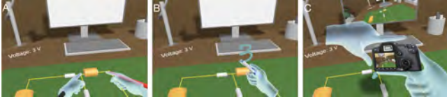
Figure 4: Hand Interfaces allow users to easily use various tools in an educational setting. Specifically, Multimeter probes are used to measure voltages, the Pen is used for writing notes, and the Camera is used for taking a photo of the current scene.
