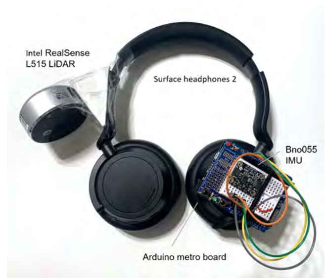
Figure 4: Wireless headphones equipped with an IMU (right) and a LiDAR (left).
