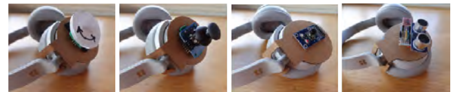
Figure 3: An early prototype showing modular customizable hardware through a hot-swappable magnetic mount.
