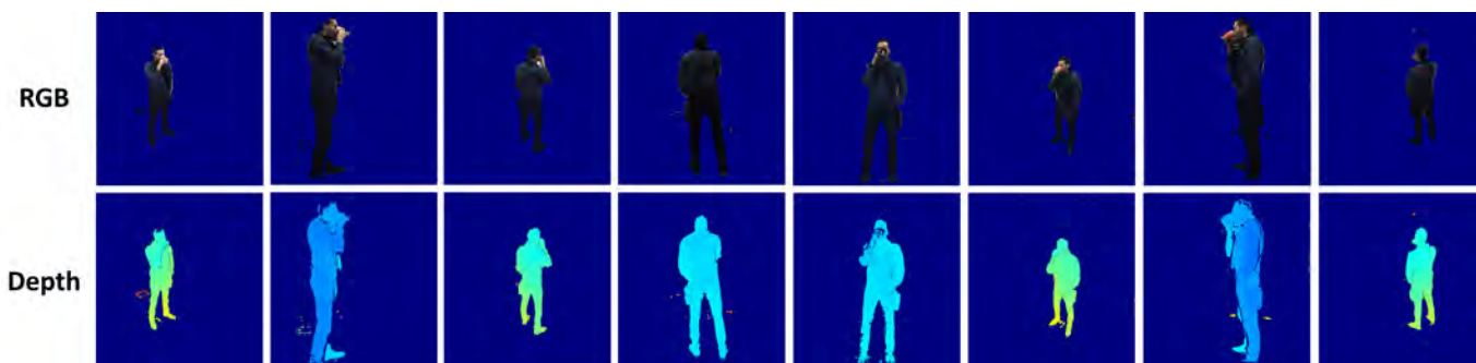
Figure 4. Top: RGB stream. Bottom: depth stream. Images are masked with the segmentation output.
