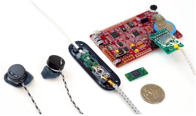
**Figure 12.** From left to right: (1) I/O Braid USB-C headphones. (2) Nano board, custom PCB for 3×3 I/O Braids with onboard tap/gesture sensing and sound tone generation. Configurable as a USB audio interface and as a USB Human Interface Device (e.g., keyboard). (3) 4×4 I/O Braid connected to a PSoC S-Series Pioneer Kit through a custom breakout board.
