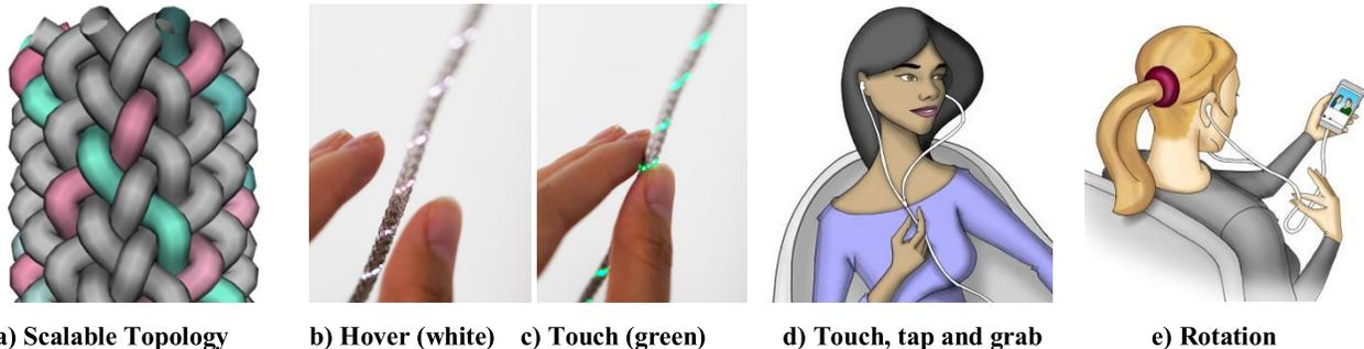
**Figure 1.** a) I/O Braid with spiraling capacitive sensing lines forms repeating 3×3 sensing matrices. b) Braided fiber optics allows integrated lighting. c) Visuals serve as feedback with intensity and color. d) I/O Braid is suitable for eyes-free interactions, as it allows rich gesture input anywhere along the cord. e) Besides touch sensing, the topology provides a robust rotation mechanism.
