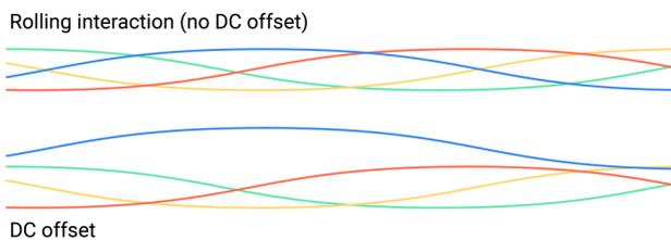
**Figure 4. The top graph shows the expected phase relationships for rolling interactions. The bottom graph shows how a DC offset for one of the signals (blue) affects the apparent phase relationships.**
