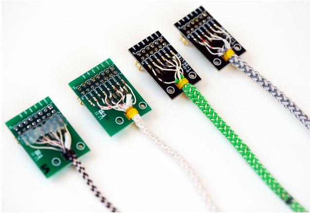
**Figure 11.** I/O Braids with different materials, texture, colors, and topologies connected to breakout boards. Black/white 4×4 (green PCB), White 4×4 (green PCB), White/green 3×3 (black PCB), Grey/white 3×3 (black PCB).
