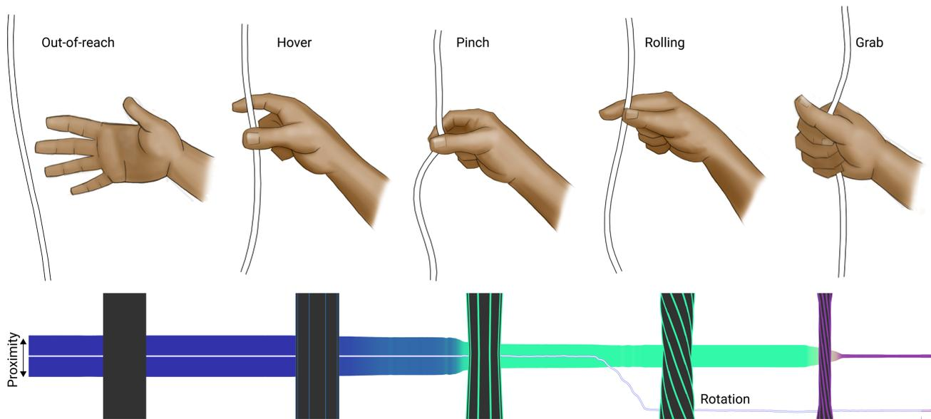
**Figure 5.** I/O Braid enables interaction techniques based on the capacitive sensing of proximity, contact area, contact time, roll, and pressure. For each event shown at the top, the bottom graph shows rotation through a center line plot, and nearing proximity by narrowing the height of the area plot. Additionally, a 3D representation of the cord is rendered at each event, with increasing line thickness for proximity, and varying thickness based on contact area.
