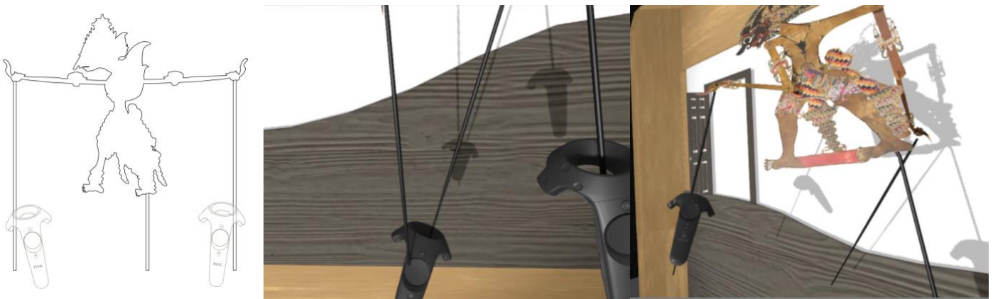
Fig. 5. principle rod puppet control scheme (left) implemented controllers and pick up functionality (middle) controlling the Wayang Kulit puppet with different hand controllers behind a projection screen (right).
