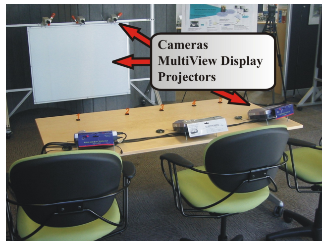
Figure 1. This photograph shows a MultiView site used in our experimental setup.
