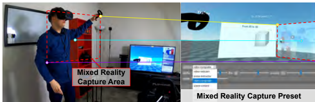
Figure 4: XRStudio implements a three-point calibration technique where the instructor first demonstrates to the system the location of the physical camera (cyan), then picks the top-left (yellow) and bottom-right (purple) corners to define the mixed reality capture area. This calibrates the position, rotation, FOV, and aspect ratio of the virtual camera. The instructor can tune each parameter so that VR representations of the controllers map the physical counterparts.
