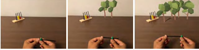
Figure 11: Output - Surface Anchored: The user can spawn the trees as the position of the token moves.
