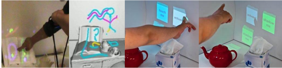
Fig. 7. Left and Center Left: Painting on any surfaces as in [10] but with coupled output. Center Right: Virtual buttons are triggered by touch if the projector is close to the surface (implying the user can reach the surface) or (Right) by shadow if the user is at a distance.
