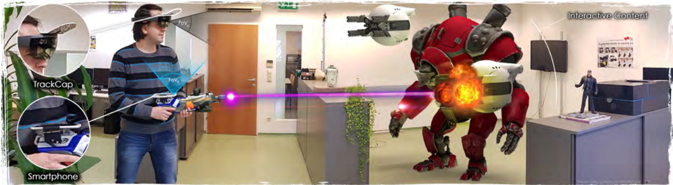
Figure 1: Our system enables using smartphones for 3D interactions in applications on head mounted displays (HMD). It consists of a planar tracking target attached to the HMD, a tracking software on the smartphone that estimates the pose of the phone relative to the HMD, and a network interface that transmits the pose to the HMD. This system enables interactions of the phone with virtual objects that are placed in world coordinates. In this example, we interact with virtual objects by attaching a smartphone to a plastic toy gun. While previous approaches require holding the device in the field of view of the HMD's camera (black), our system supports a large interaction space by using the camera on the phone for tracking (blue).
