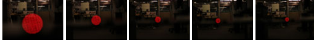
(b) Photos with the camera at increasing distances away from the barcode ( 25\text{cm} for the leftmost and 2\text{m} for the rightmost photo). The 15\mu\text{m} feature size Data Matrix codes are decoded reliably at distances up to 2\text{m} with a 85\text{mm } f/1.8 lens.
