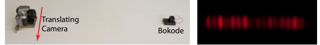
Figure 6: Capturing a 1D Bokode using camera translation. (Left) The camera translates perpendicular to the Bokode’s optical axis during the length of the exposure. The camera has a small aperture size of f/8 , the lens focuses at infinity, and the total translation is about 4cm. (Right) Resulting photo as captured by the camera.
