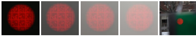
(a) Effect of ambient light on the Bokode pattern contrast. (Left to right) Increasing ambient light intensity by aiming multiple fluorescent lamps directly at the Bokode with a fixed exposure time and Bokode LED intensity. (Right most) Photo of a Bokode taken outdoors in sunlight.
