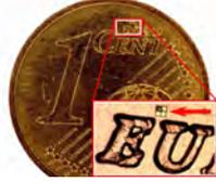
Figure A.21: Size of the sensor in comparison to a Euro cent coin. The size of the sensor is approximately 180x180  $\mu\text{m}$ .
