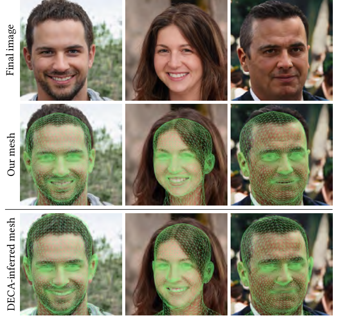
Figure 4: Top: Geometric match between the final image and the head shape and pose generated by the geometry, expression, and camera networks for three latent codes. The accurate correspondence enables responsive and intuitive control of the final image via manipulation of the 3D mesh. Bottom: Mesh inferred by DECA [Feng et al. 2021] from our rendering. The weaker correspondence (see esp. eyes and mouths) suggests that automatic geometric labeling would not be reliable in producing training targets or estimating whether the rendering follows the mesh accurately.
