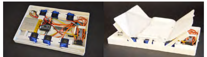
Figure 11. Shape-changing tablet containing 6 servo motors. Each corner can be bent, as well as the center of the tablet.
