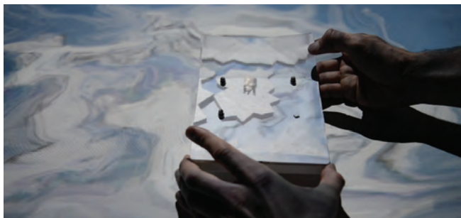
Figure 6. By rendering contents on the table, the device blends into the environment and can render apparent holes.
