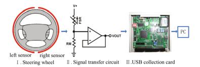
Fig. 1. Platform of detecting grip force of steering wheel
