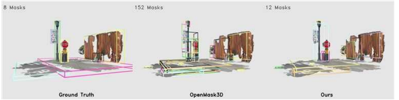
Figure 6: From left to right: bounding boxes from the ground truth, OpenMask3D [101], and our proposed method. OpenMask3D predicts a large number of masks, resulting in excessive bounding boxes that over-represent the same scene objects. In contrast, our method produces fewer, more accurate boxes. (Box colors are arbitrary and can be ignored.)
