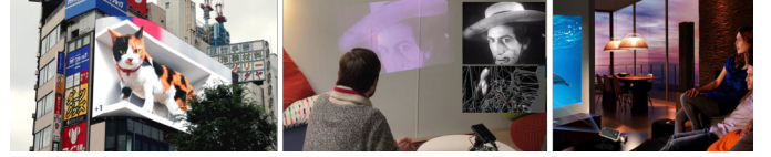
Fig. 6. Displaying virtual contents with mature technologies: Public Large Display (Left); Pico-projector attached on top of a wearable computer (Middle), and; mini-projector inside a smartphone (Right).
