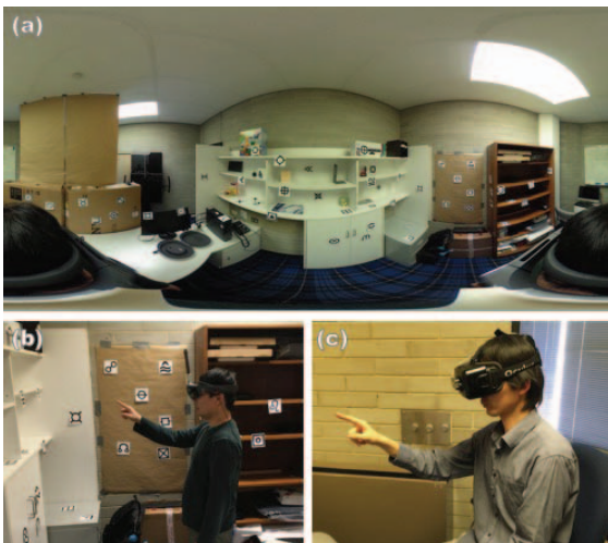
Figure 5: Experimental setup: (a) 360 panorama picture of the local host user’s space, (b) setup on the local host user’s side, (c) setup on the remote guest user’s side.
