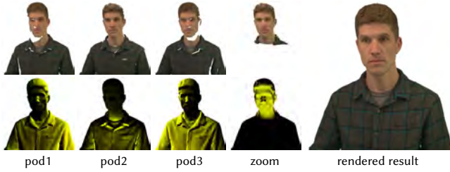
Fig. 10. We project each color image onto the fused surface and combine these using blend weights (yellow) determined from the surface normal.
