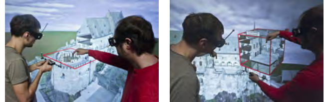
Figure 6. Two users examining interior parts of a building model with a Photoportal used as a cutting plane (left) or a 3D cutout (right).
