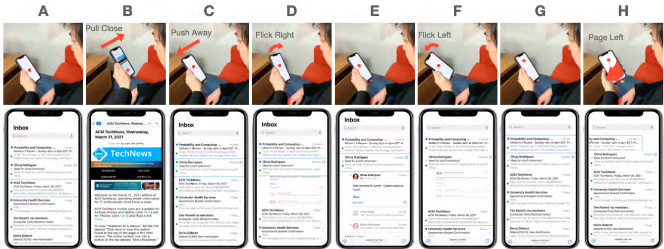
Figure 5: Email Client: A user is browsing their inbox (A). Spotting an interesting email, the phone is pulled closer to take a peek(B), and then pushed back to close it (C). An email thread’s details are unrolled with a right flick (D), and after reading (E), rolled back up with a flick left (F). Finally, an unimportant email is deleted with a page left gesture (H).
