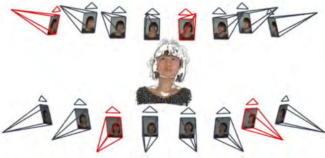
Fig. 7. Spatial layout of our camera setup. Marked in red are the 4 views used for evaluation. The point cloud reconstruction is obtained via COLMAP and used for additional depth supervision.
