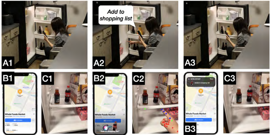
Fig. 12. In this example, a user points to a beverage and says "add to shopping list". A1-3: External reference photos; B1-3: Interface screenshots; C1-3: Views from a phone camera, unseen by the user (see also Figure 4).
