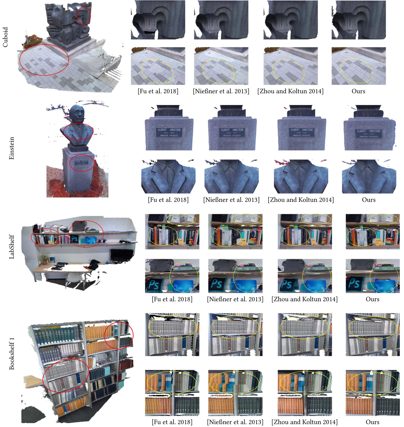
Fig. 15. Visual comparison with previous methods on various scenes of our dataset. We compare our approach against one real-time volumetric fusion system [Nießner et al. 2013] and two offline algorithms [Fu et al. 2018; Zhou and Koltun 2014]. The leftmost image of each row shows the reconstructed model by our method, and we list closeup views for models reconstructed by respective methods. Although our system operates in real time, it obtains high-quality textured meshes comparable to two offline algorithms, or preferably better in some scenes.
