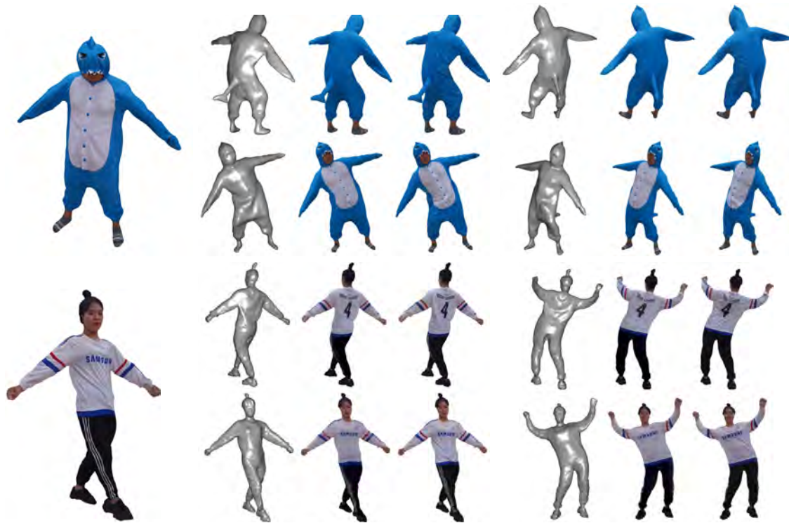
Figure 16: Additional results. (left) snapshots of texture mapped geometry. (right) rear and front views of dynamic geometries at two timestamps. Each image trio shows the underlying geometry, global texture map-based result, and our result.
