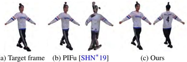
Figure 11: Comparison with a learning-based method. Textures for the target frame (a) are reconstructed by PIFu (b) and our method (c). In PIFu, the input is a single RGB image with low resolution. The reconstructed textures are blurry (b left) for the visible regions in the input, and contain artifacts (b right) for the invisible regions.
