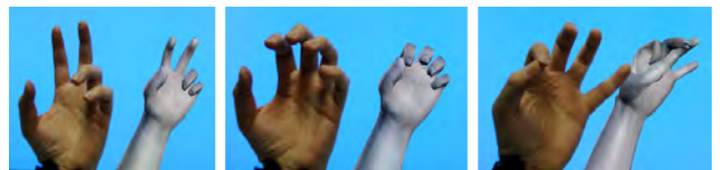
Figure 12: Truer hand pose recovery with inverse kinematics. Note PIP and MCP joint angles recovered correctly.
