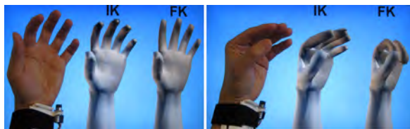
Figure 15: Failure cases for our forward kinematics (FK) model. Notice mismatch in PIP angle (left) and MCP angle (right). Using our inverse kinematics (IK) model we can mitigate such issues, and offer a truer reconstruction.
