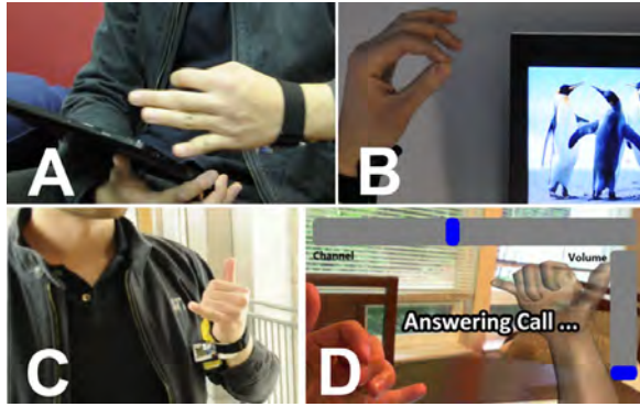
Figure 4: Digits application scenarios. A+B) Extending interaction space around a mobile device into 3D. C+D) Non-visual UIs allow users to manipulate application parameters without looking at or touching a physical device (GUI elements are for illustration only).
