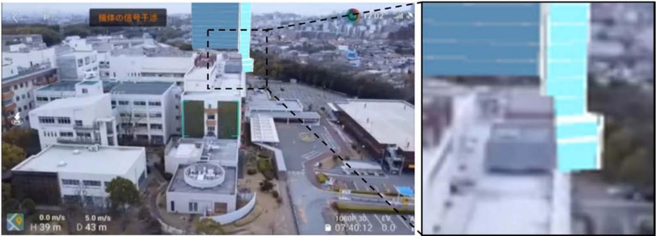
Figure 25: Incorrect occlusion handling in the site A field test ( $40 \pm 1$  m altitude).
