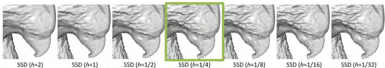
Fig. 9: Reconstruction of the noisy Eagle dataset ‡ using the Smoothed Signed Distance reconstruction [Calakli and Taubin 2011] using various settings of the Hessian weighting parameter ( h ). (The highlighted results are those with the default parameters used for evaluation in Section 6.1.)
