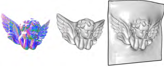
Fig. 3: Reconstructions of the Angel point set ‡ (left) using Dirichlet (center) and Neumann (right) boundary conditions.
