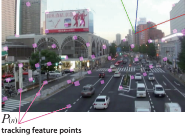
Figure 3. Generation of out-of-body view: it virtually constructs wider view from first-person video on basis of SLAM.
