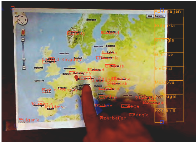
Figure 2. Access Lens viewing a map. Touching near the map labels speaks their names. An edge menu along the right edge of the page shows a sorted index of on-screen items.
