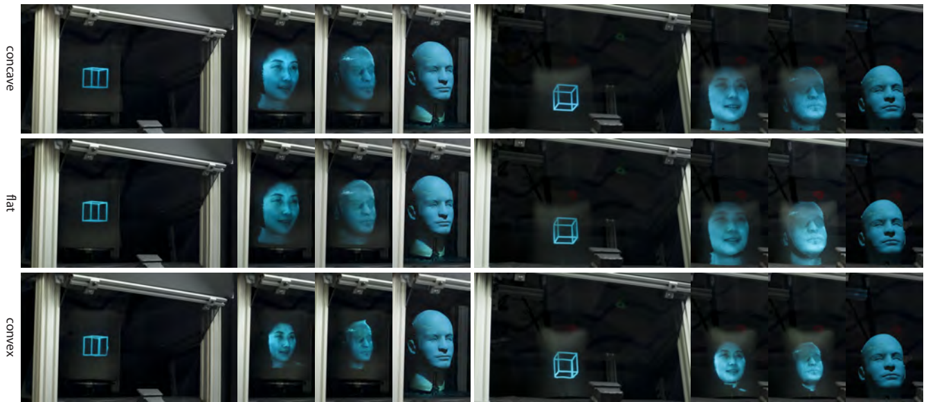
Figure 10: Comparison of the different mirror shapes for simultaneously tracked upper and lower views. (Row 1) Concave mirror (Row 2) Flat mirror (Row 3) Convex mirror. For the convex mirror, the geometry was scaled by 0.75 to fit within the smaller display volume. In the 4th and 8th columns we replaced the mirror with the actual mannequin head to provide a ground truth reference.
