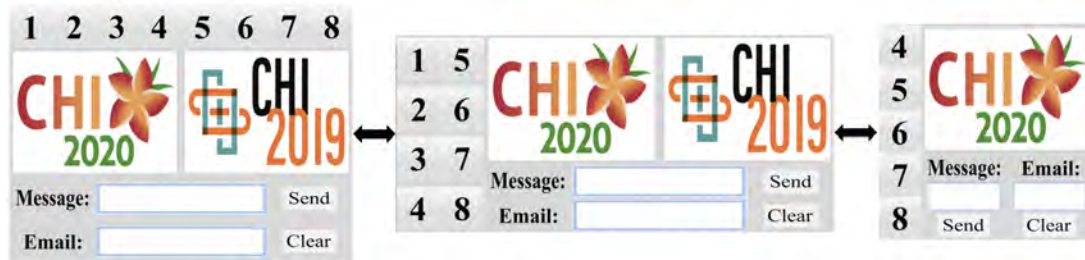
Figure 1. ORCSolver is able to adapt a layout between different sizes and orientations at near-interactive rates, based on a single layout specification. The layout is adjusted to fit the aspect ratio, and the optional “CHI2019” logo and buttons 1, 2, 3 are automatically removed as space gets scarce.
