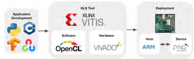
Fig. 8. Example of FPGA implementation flow using HLS tools presented in [36].
