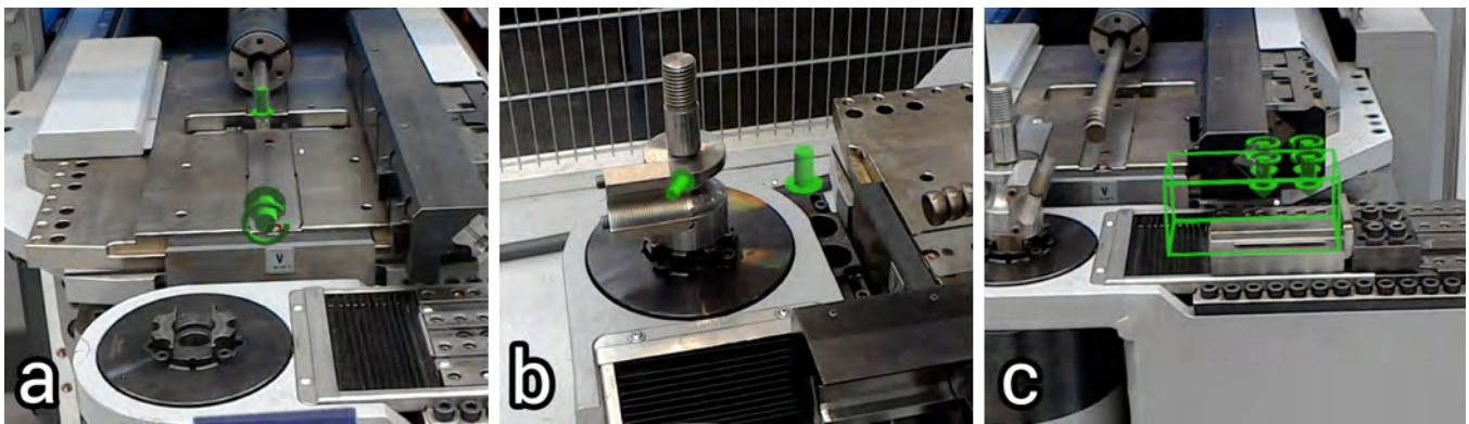
Figure 3: Abstract AR visualization of assembly step a) 1, b) 7, c) 11.
