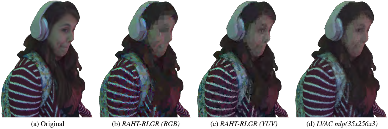
Figure 13. Subjective quality around 0.25 bpp. (a) Original. (b) 0.258 bpp, 24.6 dB. (c) 0.255 bpp, 25.9 dB. (d) 0.255 bpp, 28.0 dB.
