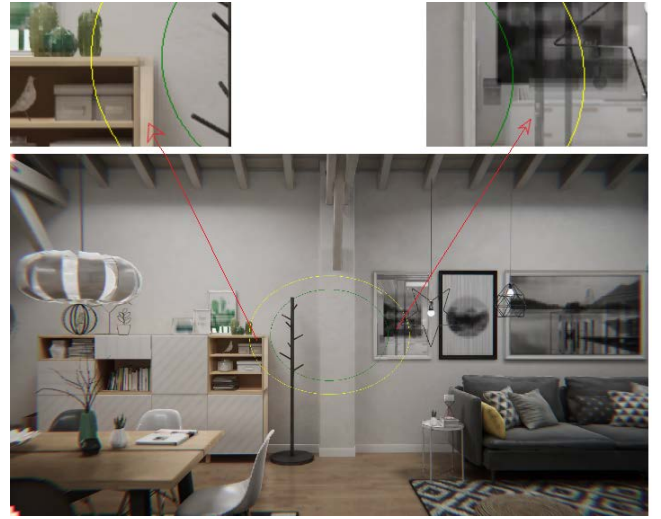
Figure 2: Frame rendered with three shading rates: one shading pass per pixel (inside green ellipse), per 2x2 pixels (between green and yellow ellipses) and per 4x4 pixels (rest).
