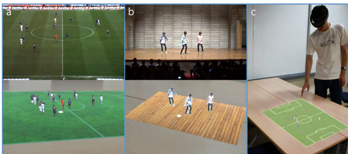
Figure 1. MonoMR enables users to easily synthesize pseudo-2.5D mixed reality content from monocular videos uploaded on the Internet or taken with common imaging equipment such as smartphones and cameras. With the MonoMR system, the user can create and experience immersive mixed reality content from various monocular videos, such as (a) sports broadcasting videos and (b) entertainment videos. (c) The synthesized content can be displayed in the real world through a mixed reality head-mounted display.
