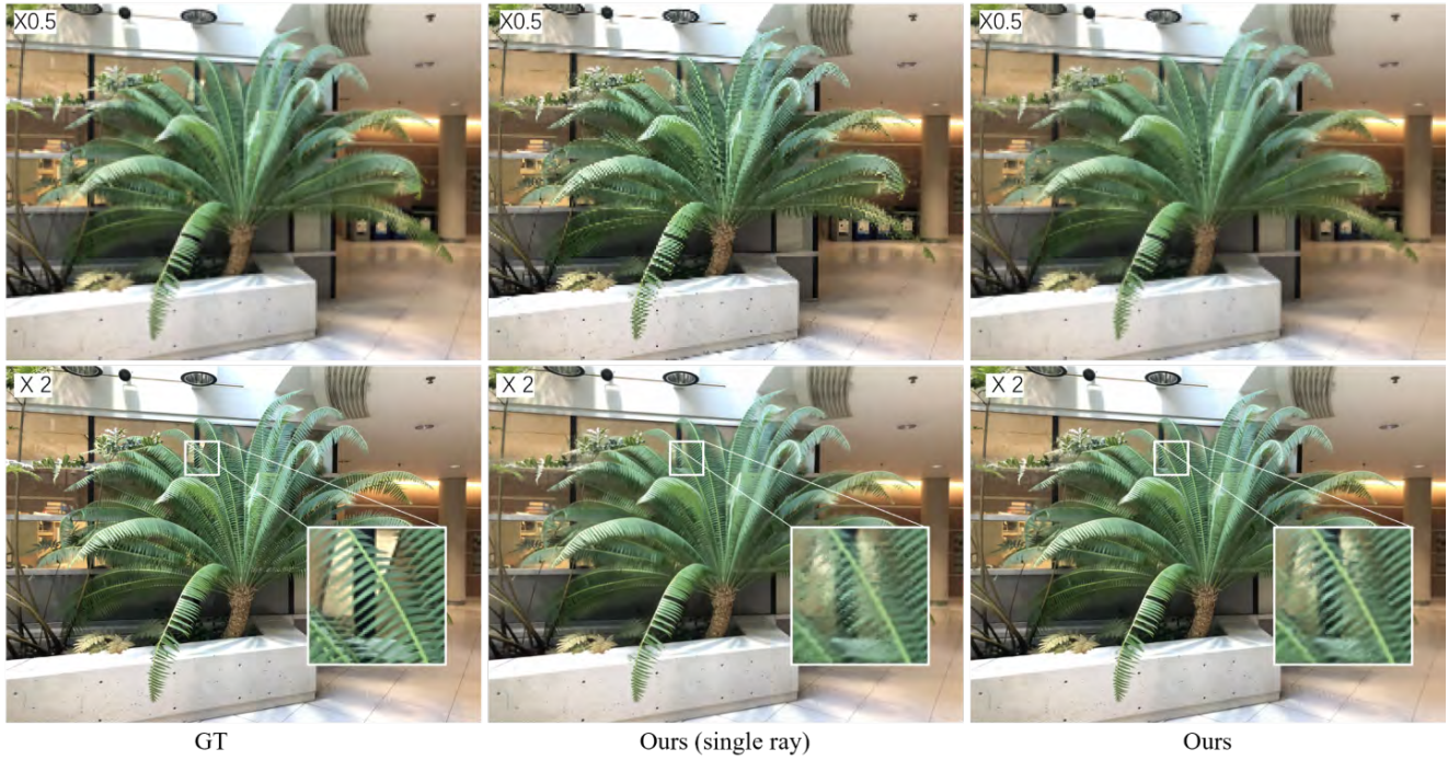
Figure 10. The qualitative results of our model that renders a pixel from a single ray. The top row shows the novel views rendered at \times 0.5 scale. Our model (single ray) produces aliased novel view. The bottom row shows the novel views rendered at \times 2 scale. Our model (single ray) produces novel view with artifacts at thin structures.
