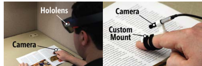
Figure 1. Prototype HoloLens and finger-camera system: (a) reading a magazine article; (b) close-up view of the camera.
