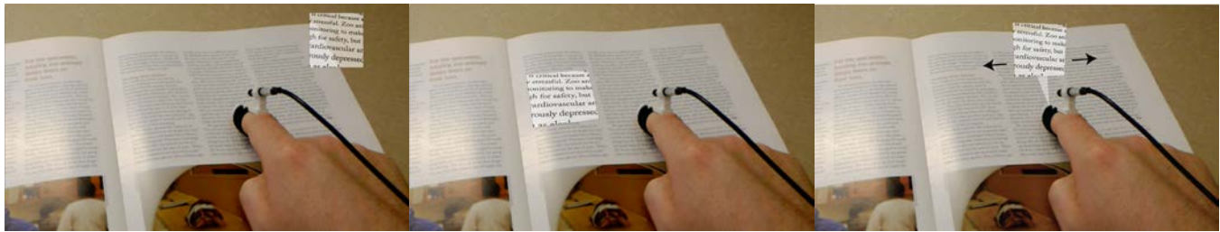
(a) Fixed position on 2D AR display ( i.e. , fixed within the wearer's field of view). (b) Fixed position on 3D surface or midair, in this case rendered flat on the magazine page. (c) Dynamic finger tracking, where magnified view follows and hovers above the finger.
