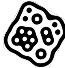
Figure 5.5: A reactIVision fiducial. The specific pattern of the paper marker ( id = 0 , angle = 30^\circ ) is recognized by the reactIVision vision engine with the aid of a web camera.
