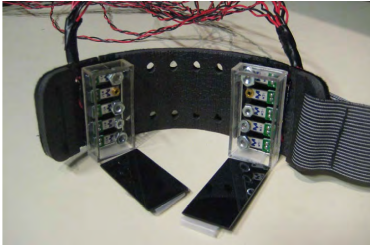
Figure 2.3: The Skinput prototype armband. Two arrays consisting of five vibration sensors each capture vibration of flesh and bones caused by touch.
