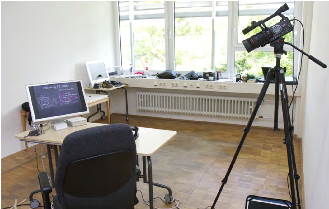
Figure 4.2: Study setup for the Wizard of Oz study. From her workspace (table, foreground), the user had an unobstructed view on all objects (background). Object manipulation for solving the tasks (displayed on the monitor) was captured by two cameras to the left (beneath the monitor) and right).
