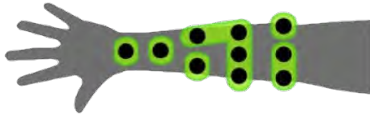
Figure 2.4: Input accuracy achieved by Skinput. Worn above the elbow, the sensor can distinguish six touch zones on the user's forearm featuring a touch detection of true positives by 88,8%.
