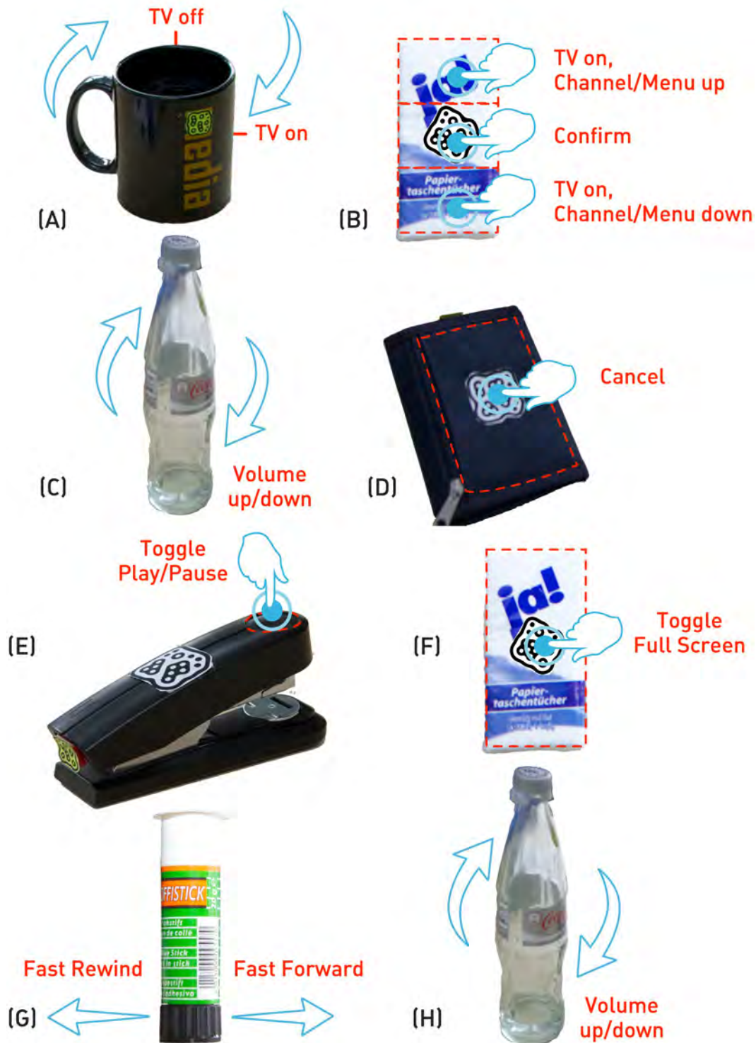
Figure 5.14: Predefined gestures for appropriated objects. (A) – (D) show the object-gesture mappings for the TV scenario. The cup handle, for instance, was meant to be turned to twelve 'o clock position for turning the TV off; turning the handle to two/three 'o clock position switched the TV on. (E) – (H) illustrate the mappings for movie player control. Red dashed shapes separate touch-sensitive regions.
