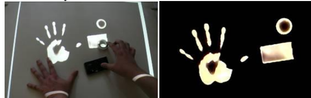
Figure 1: The capabilities of a liquid displacement table. Left: the user pressing a hand, cellphone and tape roll onto the surface to interact. Here the objects cause the black liquid to be displaced as the white latex is pressed onto a sheet of acrylic. This produces a bright white imprint of the objects, which is captured by a camera placed underneath the surface. Right: the raw unprocessed images as captured by the camera. These are also projected onto the surface from above. Note that the approach requires near zero force to interact, and that objects can be sensed at speed in full motion.
