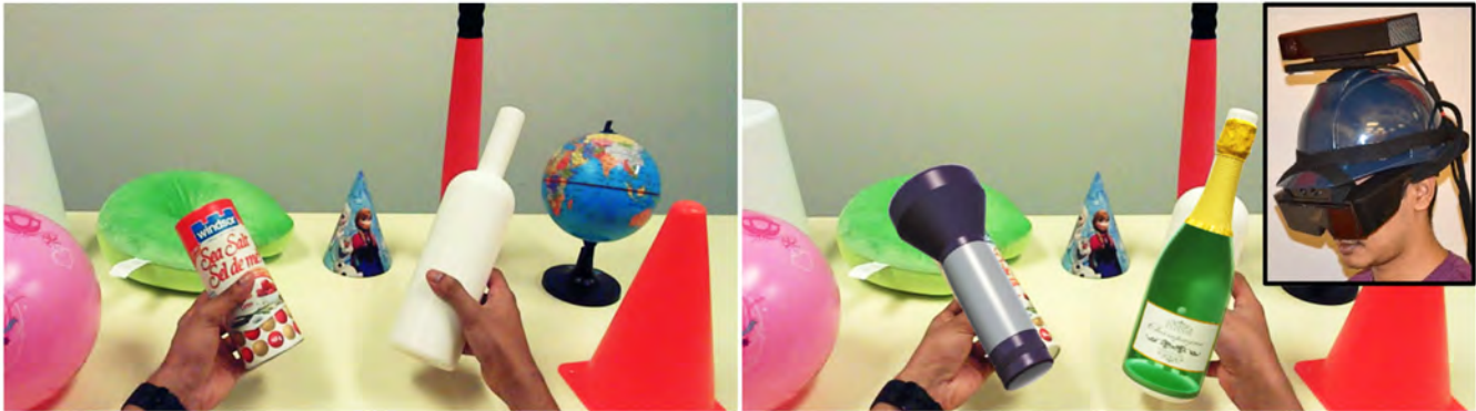
Figure 1. Left: a user's table as seen un-aided by augmented reality. Right: The same user's table, as seen through our AR headset, augmented with our Annexing Reality tool. Note that virtual content is placed and scaled in order to opportunistically take advantage of physical objects in order to provide haptic experiences for virtual ones.
