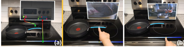
Figure 8: Virtual video tutorial controller: (a) The continuous electric range edge is connected to a progress bar and the discrete pan handle edge is connected to a ‘play/pause’ behavior. (b) The user can click on the handle of the pan to start/pause the video and utilize the range edge to jump to the next part.
