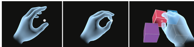
Figure 3. A white cursor located near the virtual hand (left) indicates where the hand will grasp an object (middle). If the cursor is inside the object, then the user can grab it (right).
