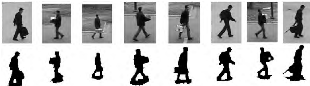
Fig. 17. (a) Example of people carrying an object and (b) the foreground regions detected by background subtraction.
