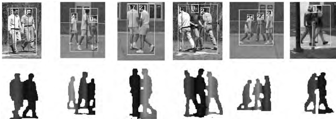
Fig. 27. Examples of person segmentation applied to foreground regions in a single image.
