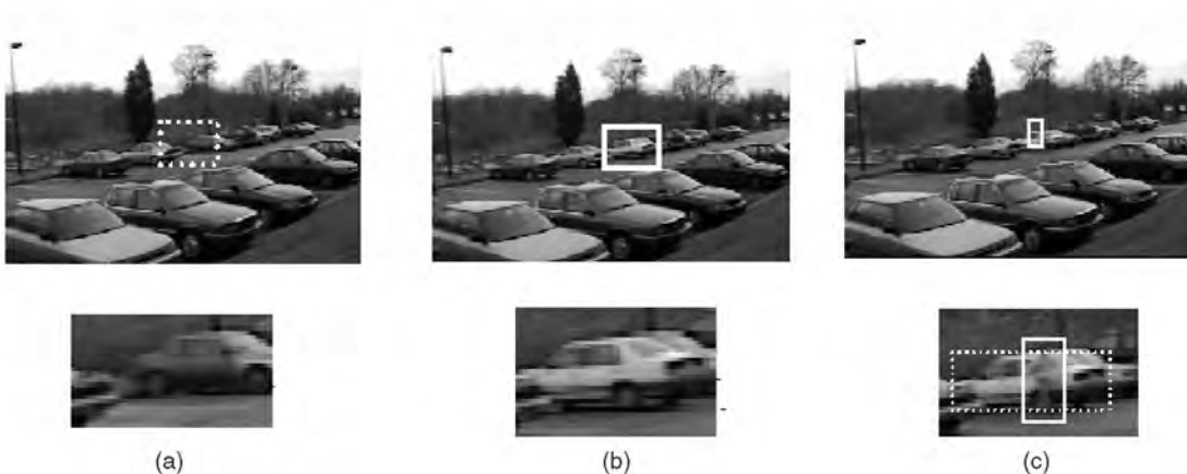
Fig. 4. A car which has been parked for a long time is added to background models (a) and (b), so the person getting off the car is detected (c).
