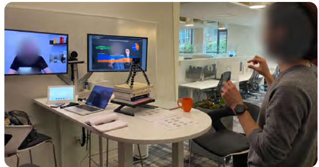
Figure 7: In the presenter evaluation, a webcam (mounted on a tripod placed at the center of the table) captures a participant’s hand motions while chart overlays on their video appear in the right monitor; a researcher assuming the role of the remote audience appears in the left monitor.
