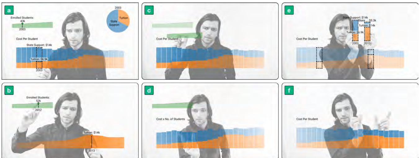
Figure 4: Coordinating and manipulating overlays: linked highlighting across charts (a) can be superseded with (b) bimanual pointing; (c) pinching and dragging a cloned copy of the green student enrollment area chart; (d) releasing the cloned area chart over the cost-per-student bar chart (which shares the same temporal domain) multiplies corresponding values, yielding total cost values over time; (e–f) pinching generates ephemeral and draggable cloned elements for spatially-adjacent comparisons.
