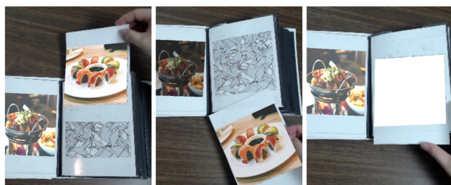
Figure 6. Tangible Album Interaction: Removing a photo. The user first removes the marker by sliding it out from the top, then reinserts it from the bottom, resulting a blank augmented photo indicating photo deletion. The reinsertion ensures that other linked digital albums are not affected.
