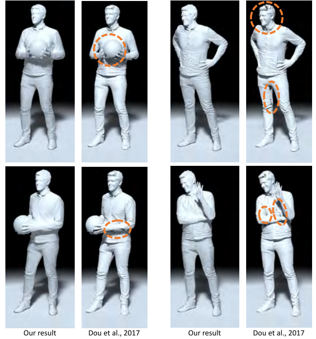
Fig. 18. A comparison of our reconstruction with Dou et al. [2017]. Note that our reconstructions are complete while holes (circled) remain with the approach of Dou et al. [2017].
