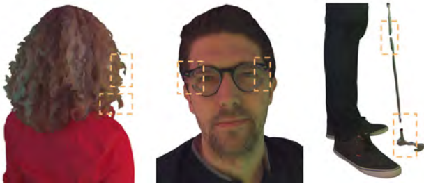
Fig. 24. Our system struggles to reconstruct the geometry of some thin structures (hair), and also transparent and highly specular surfaces.
