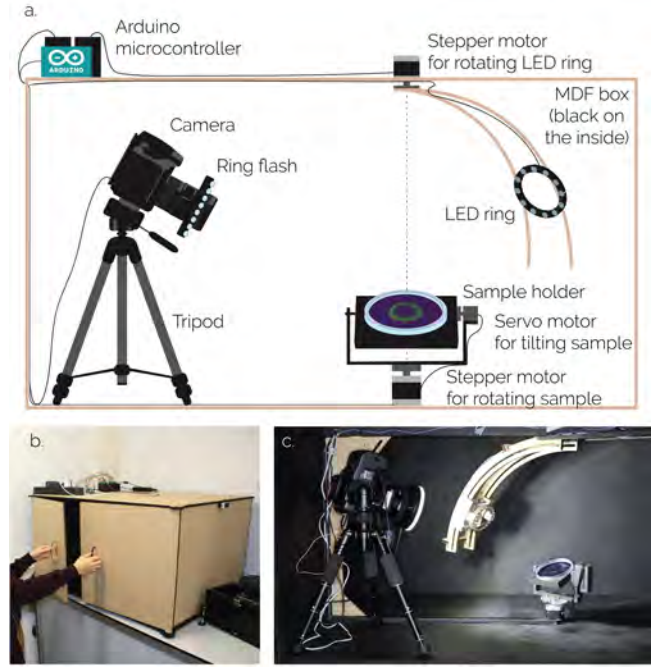
Figure 6: The capture tool. (a) Infographic of the capture tool. (b-c) The protective MDF box from the outside and inside.
